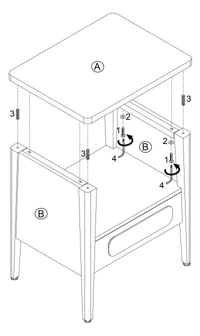
Fully tightening everything to 100%. Ensure all legs are touching the ground by using Leveler.
