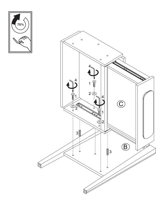
Repeat Step 2 for the remaining Leg Frame (B), also tightening to 75%.
