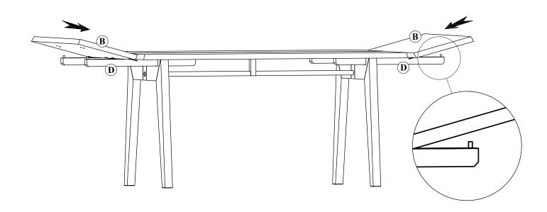
Attach the Extension Support Rail (D) to the Top Extension Leaves (B). Using the Plastic Head Bolts (1) and Flat Washer (5) removed from step 12 Tighten to 100%
