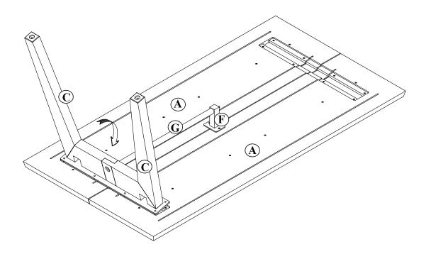
Using the Bolt (2), the Lock Washer (4), the Flat Washer (5) and the Allen Key (7). Tighten to 100% Then use the Bolt (3) and the Allen Key (7). Tighten to 100%
