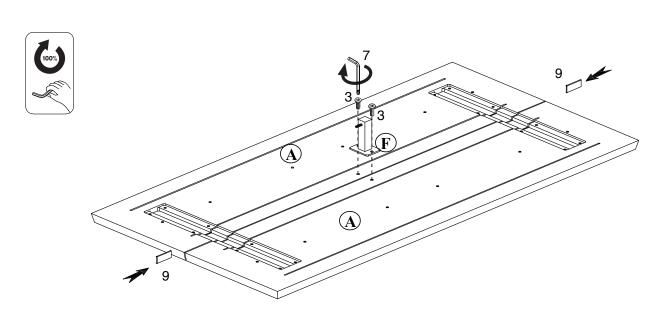
Attach the Metal Support Bar (G) to the Metal connector (F) Tighten to 100%
