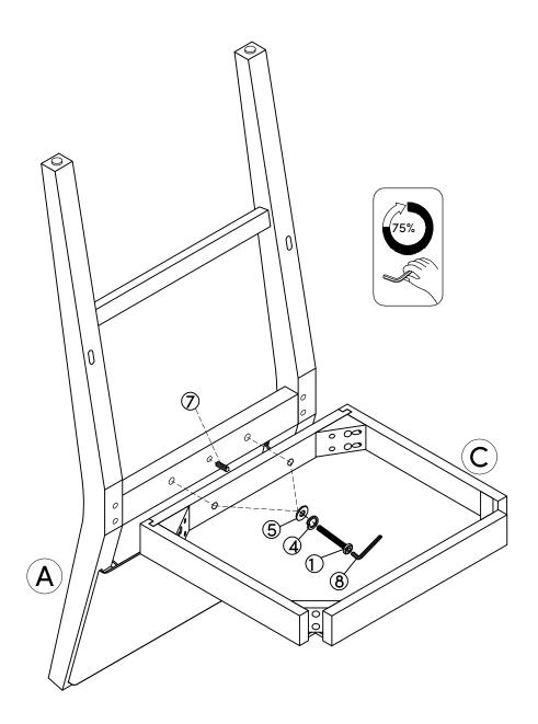
Let's secure those legs in place! Secure using the Flat Washers (5), Lock Washers (4) and Hex Button Head Bolts (3). Tighten to 75% using the Allen Key (7).
