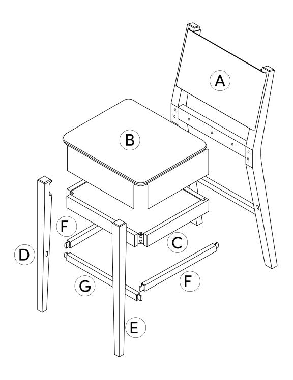
Secure on the Chair Back (A) and the Seat Frame (C) using the Flat Washer (5), Lock Washer (4) and Hex Button Head Bolt (1). Tighten to 75% using the Allen Key (7).
