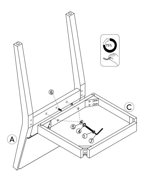
Let's secure those legs in place! Secure using the Flat Washers (5), Lock Washers (4) and Hex Button Head Bolts (3). Tighten to 75% using the Allen Key (7).
