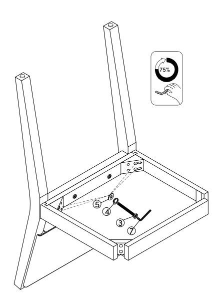
Secure on the Front Legs (D) and the Seat Frame (C) using the Flat Washer (5), Lock Washer (4) and Hex Button Head Bolt (2). Tighten to 75% using the Allen Key (7).
